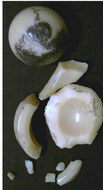
4.11.2010: 1. revision: CoCr head and PE Anca inlay
